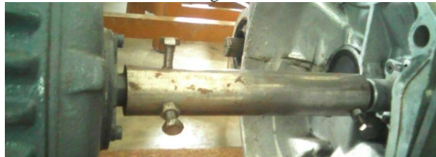
Fig.5: shaft coupled to motor and gearbox
